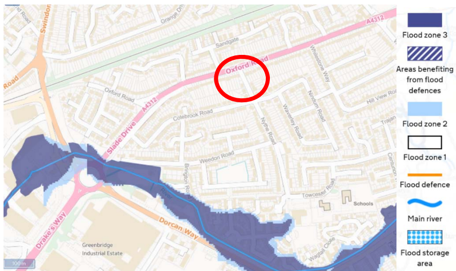
Figure 3-9 Flood Zone Map of Area Surrounding Oxford Road/Nythe Road Junction
