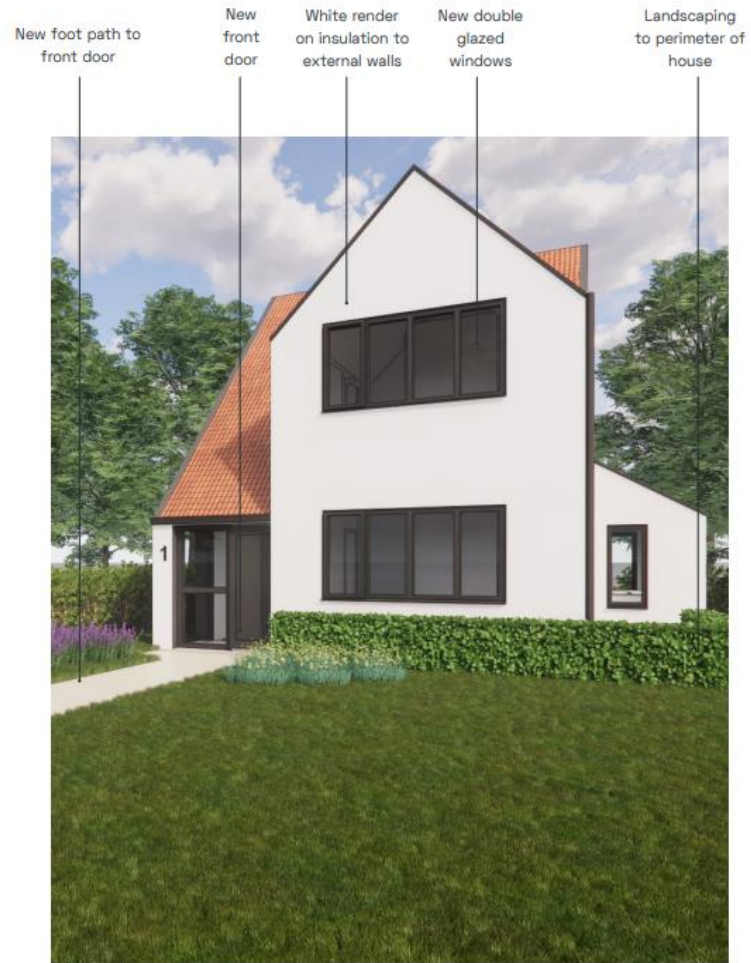
3D View showing the proposed upgrades
